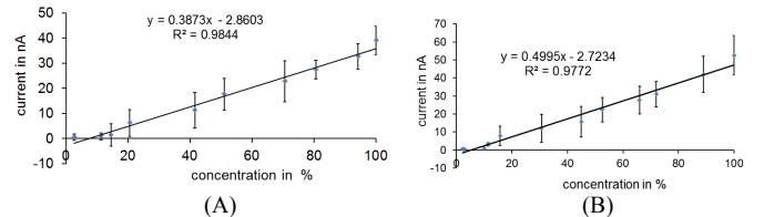
Fig.4. Calibration curve: (A) with Nafion and PCTE membrane; (B) with Nafion but without PCTE membrane.
