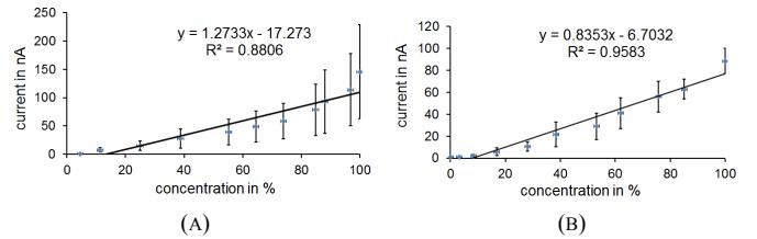
Fig.3. Calibration curve: (A) without electrolyte and membrane; (B) with 0.1M KCL electrolyte and PCTE membrane.
