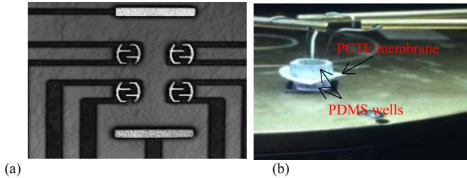
Fig. 1. (a) microphotographs of the microelectrodes used. (b) Close-up view of experiment setup with membrane and PDMS well.
