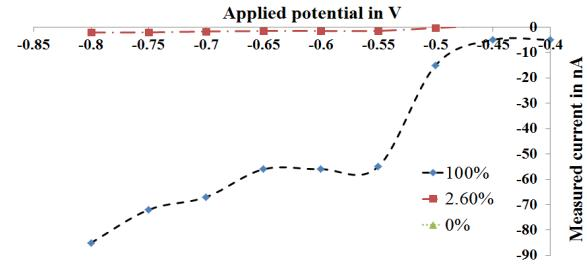
Fig.2. Amperometry measurements at a WE vs. RE voltage range between -0.4V and -0.8V.
